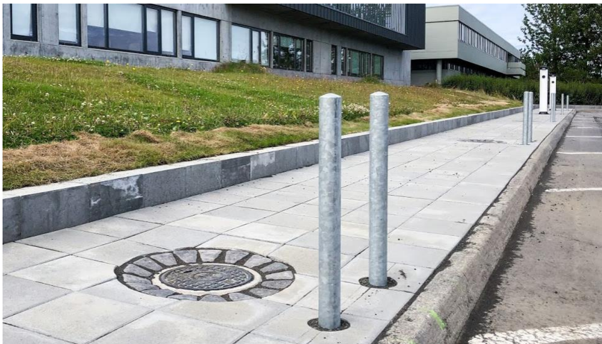
A charging ready street in Reykjavik, Iceland showing 3 future proof, scalable, pre-prepared Unimi-1bases with crash protections. In the distance, two installed EV charging stations serving current EV charging demand
